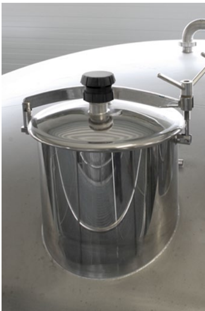
Pressure compensation valve on top of a tank
